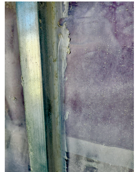
Fig. 5. A shotcrete test panel with shear wall infill confirmed that proper protection of the plaster and concrete consolidation around the stud flanges was consistently achievable.
